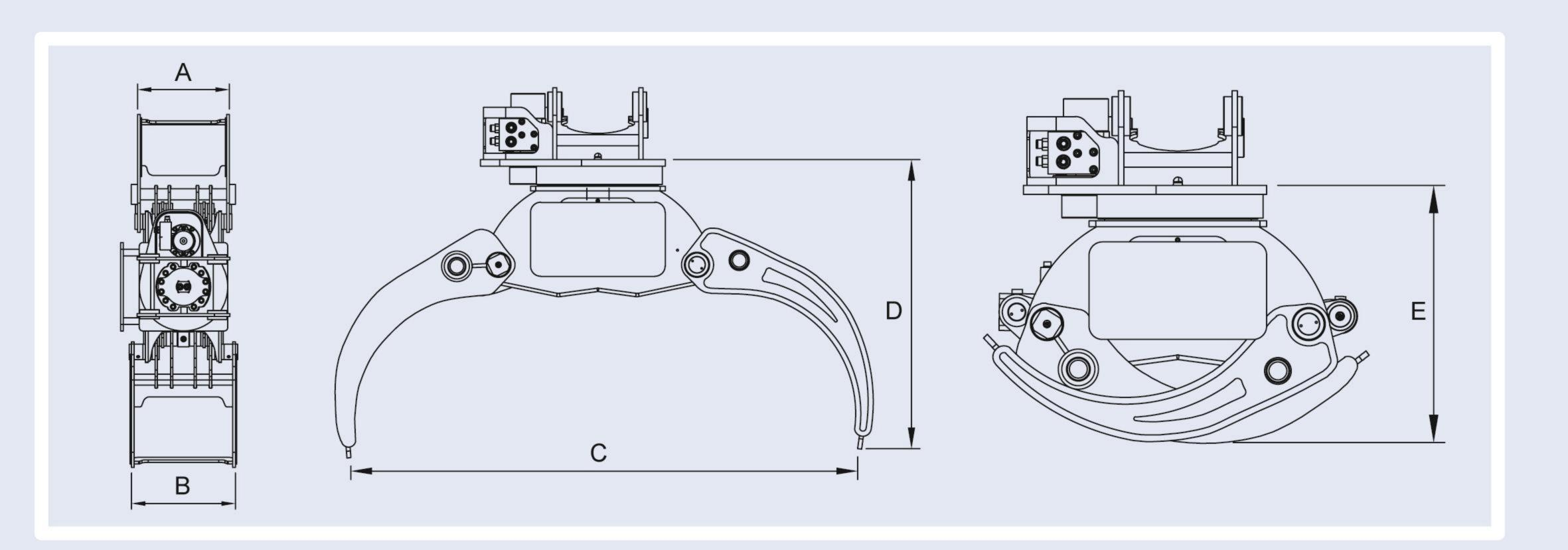
The single-cylinder and double-claw linkage mechanism can accurately grab small items such as logs and sugarcane with high grasping efficiency.
